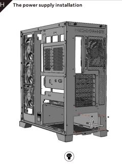
The power supply can be fixed by aligning the screw in the figure to the hole position Note: different types of power supply, hole location may be slightly different, take the actual object as the standard
