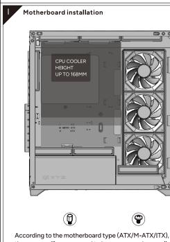
According to the motherboard type (ATX/M-ATX/ITX), the copper pillars may need to be re-arranged manually according to the fixing locations specific to your motherboard CPU Height limit: 168mm
