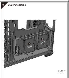
Align the SSD holes and fix them with screws.
