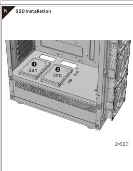
Align the SSD holes and fix them with screws.
