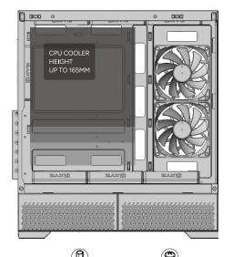
According to the motherboard type (ATX/M-ATX/ITX), the copper pillars may need to be re-arranged manually according to the fixing locations specific to your motherboard CPU Height limit: 165mm
