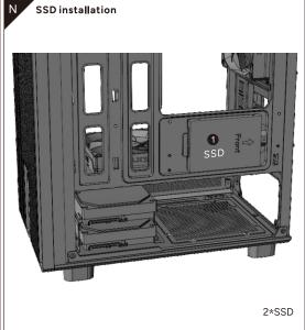
Align the SSD holes and fix them with screws.
