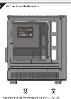
the copper pillars may need to be re-arranged manually
