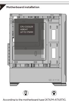
the copper pillars may need to be re-arranged manually
