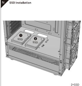
Align the SSD holes and fix them with screws.
