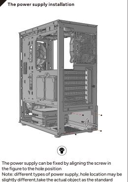
The power supply can be fixed by aligning the screw in the figure to the hole position
