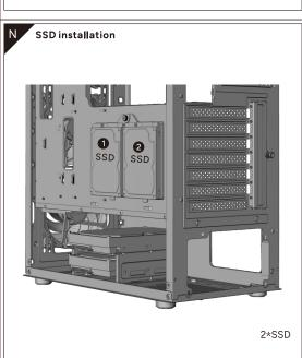
First fix the hole position with the hard disk cushioning pad,
